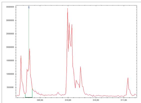
*Fe quadruplet, spectral lines 309.9897nm, 309.9971nm, 310.0304nm and 310.0666nm. The spectrum was acquired with spark excitation using the M266 with 1800 lines/mm grating. The possibility of resolving at least 3 peaks demonstrates high optical quality of the instrument.*
